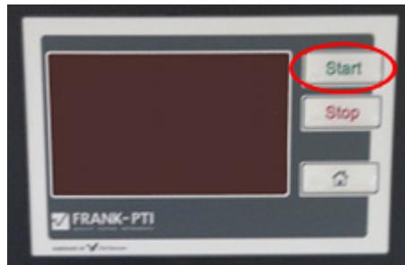
To start the measurement, press the button Start.
